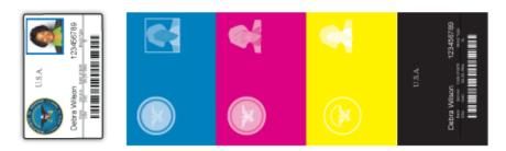
This illustration shows the same printed card and the ink ribbon used to print it, after using the Security Erase feature.
