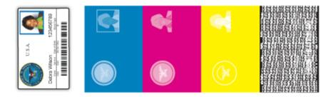
This illustration shows the retransfer ribbon after using the Security Erase feature.
